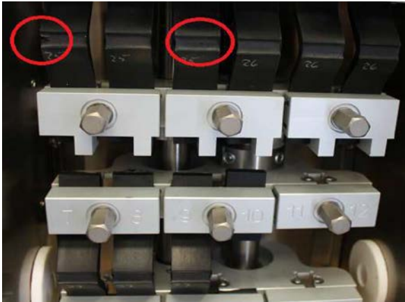
Picture 1: De Mattia test specimen after approx. 64.000 cycles operated at 160 °C
